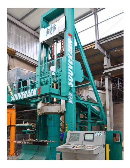
New BFS-ideas-additional benefits for our clients. The BFS-liner insertion installation can be integrated in new and existing concrete pipe machines. As an additional option it supplements the scope of a BFS-SOUVERAEN-installation.
