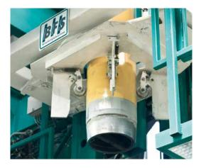
ECORESIST By the combined control of the pipe machine and liner installation the stepping order of the system is perfectly interlocked. As soon as the mould with the green pipe rotates to the insertion station, the polymer pipe is pressed in from the top.
